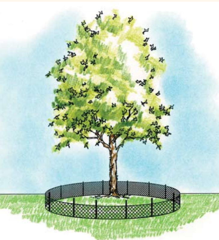
Figure 4. Protective silt fence located beyond tree's dripline.
